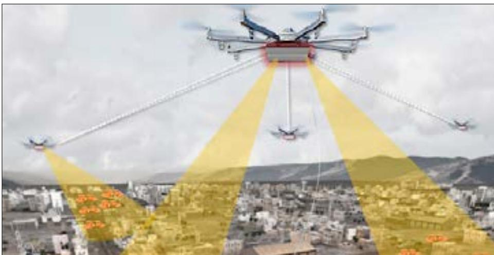
*The U.S. Defense Advanced Research Projects Agency's Aerial Dragnet program seeks to develop networks of tethered drones that can detect and track every small unmanned aircraft operating within a large coverage area, such as a whole city. Initially, such a system would be used in active battlefield environments, but the agency has suggested that the same technology could also be used for unmanned aircraft traffic management domestically.*
